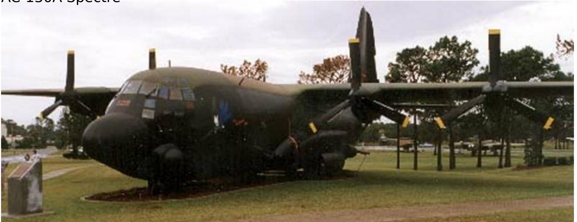
The A-model gunship was the first AC-130 model. The aircraft is 97 feet 9 inches long and 38 feet 3 inches tall. It has a wingspan of 132 feet 7 inches and a wing area of 1,745 sq. feet. Initially, the C-130 had a maximum speed of 384 mph and an un-refueled range of 2,450 miles with maximum load. However, with the aerial refueling modification, the range for the later model gunships was only limited by crew endurance.
